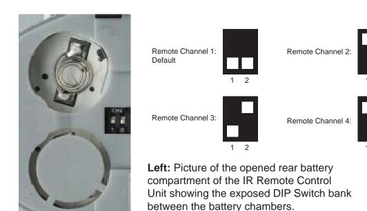
The IR channel selected on the IR Remote Control unit must match the IR channel assigned to the 2x4 Switcher for HDMI 1.3. For example, if you set both DIP switches on the remote to the down position (IR channel 1), you must set the 2x4 Switcher for HDMI 1.3 to use IR channel 1.
