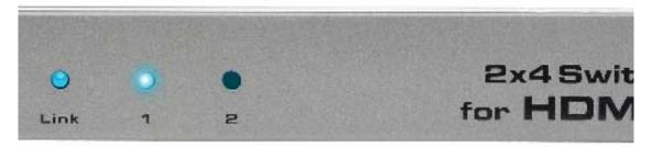
In the illustration above, the LED for Input 1 is blinking and the LED for Input 2 is inactive. This indicates that the Switcher is set to IR channel 1.
