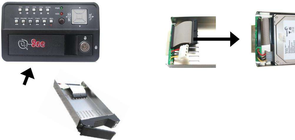
**CAUTION:** The wedge at the end of the cartridge handle must be fully inserted into the compartment; otherwise the cartridge will not be able to insert into the DVR firmly, it could also cause damage by scraping the body of the DVR.
