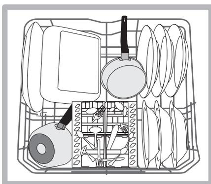
Very soiled dishes and pans should be placed in the lower rack because in this sector the water sprays are stronger and allow a higher washing performance.
