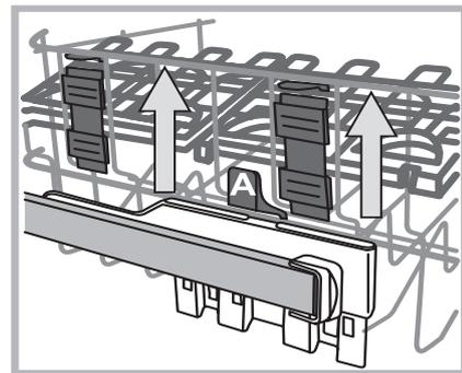
If the rack is equipped with a **Lift-Up device\*** (see figure), lift it up by holding its sides. To restore the lower position, press the levers (A) at the sides of the rack and follow the rack down.
