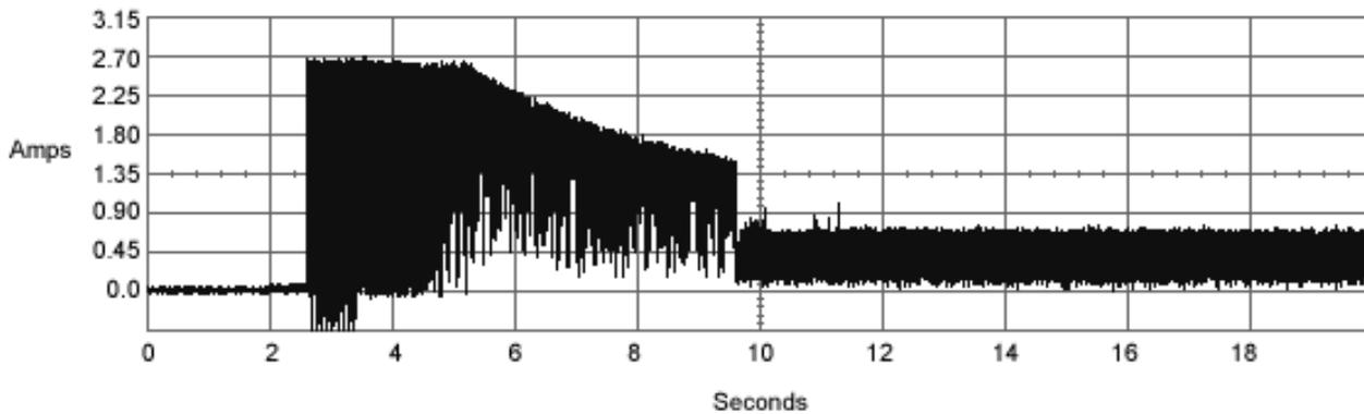
Figure 2. Typical 12V startup and operation current profile
