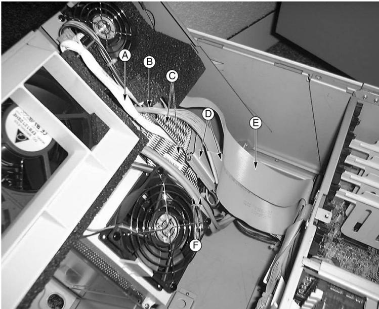
Figure 9 - Cables to the subchassis
