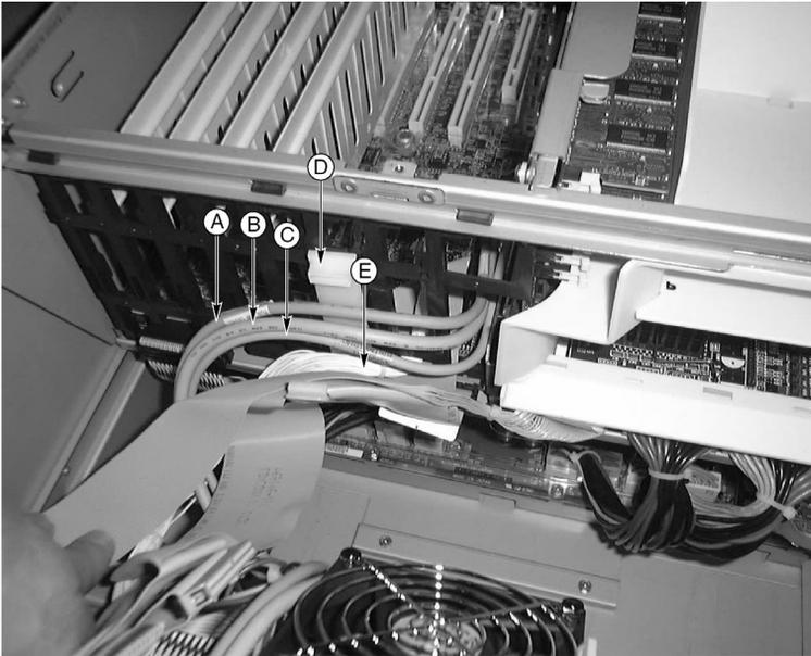
Figure 11 - Rear cables in the cable clamp
