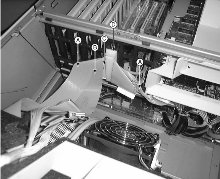
Figure 10 - Front cables in the cable clamp
