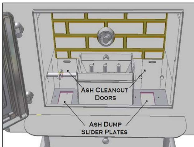
The ash dump slider plates can be opened allowing the ash and debris that has accumulated in the combustion chamber to be brushed and scrapped down into the ash pan. This can be accomplished as needed, until the ash pan begins to fill. Once the ash pan starts to fill, remove the ash pan and dispose of the ashes in a safe and environmentally friendly manner. See "Ash Disposal".
