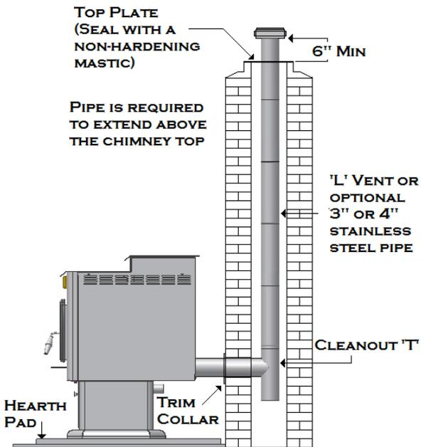
Connect the horizontal pipe by pushing it through the hole in the masonry and lining it up with the branch in the tee. Push the pipe into the tee while twisting it to lock it into the tee. If desired, once the horizontal pipe is in place, the space between the pipe and masonry may be filled with high-temperature grout.
