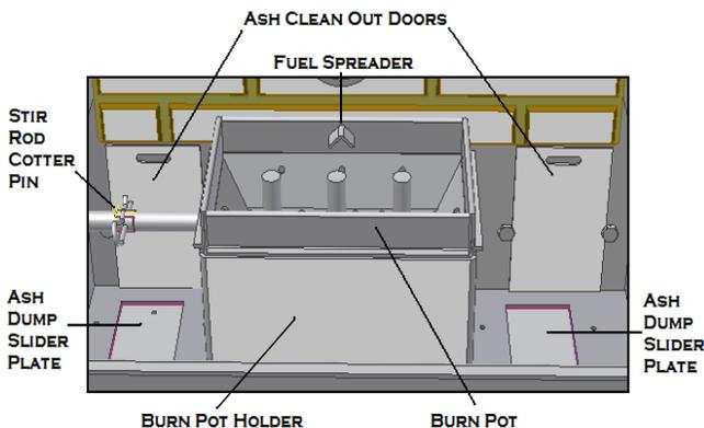
**STIR ROD & BURN POT INSTALLATION:** The Burn Pot must be set into the Burn Pot Holder with the fuel spreader towards the rear of the stove, as shown.
