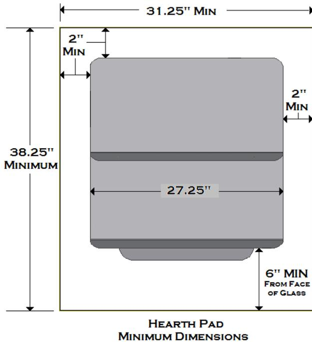
Freestanding installations require a minimum 33 1/4" wide by 36" long floor protection. The stove must be placed on a continuous (grouted joints) noncombustible material such as ceramic tile, cement board, brick, 3/8" millboard or equivalent, or other approved or listed material suited for floor protection.
