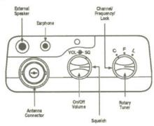
EXTERNAL SPEAKER JACK When using an optional External Speaker system, connect the External Speaker plug here.
