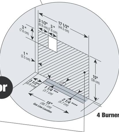
\*\*Note: Drill on centerline 1/4" from rear wall for gas supply line.
