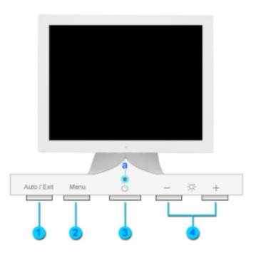
1. Auto button / Use this button to auto adjustment direct access. / Use this button to Exit the active menu or the OSD.
