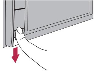
When you release your finger, the bottom of the detachable faceplate separates slightly from the navigation system.
