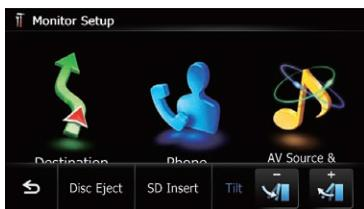
The LCD panel opens, and the disc is ejected.
