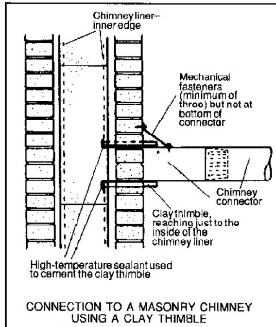
**Venting to a Masonry Fireplace Chimney**
