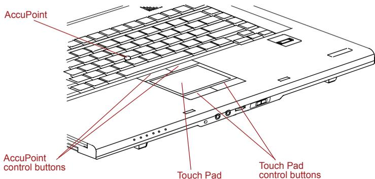
*Figure 4-1 Touch Pad and Touch Pad control buttons*
