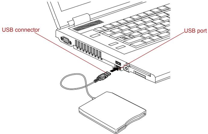
Figure 3-12 Connecting the USB floppy diskette drive
