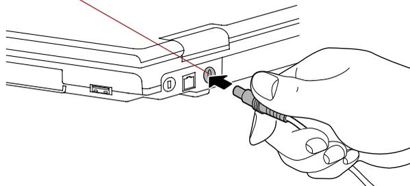
*Figure 1-3 Connecting the adaptor to the computer*
