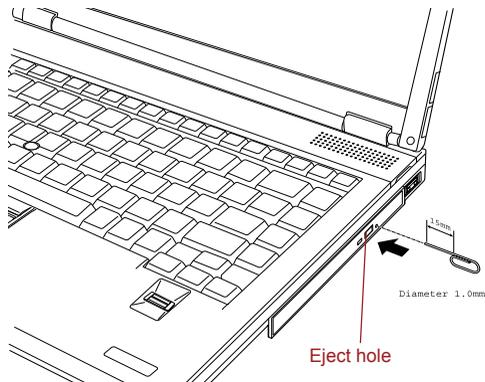
Figure 4-8 Manual release with the eject hole
