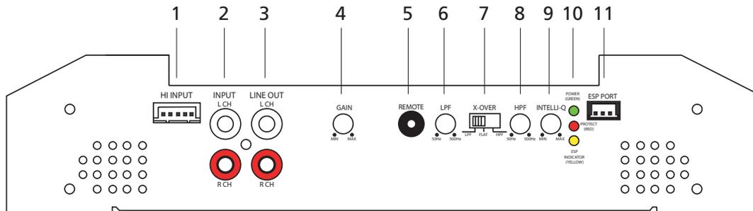
1. **Hi Input** (high level input) - Accepts 1v to 10v input from the head unit's speaker output. The amplifier will automatically wake-up when the input is greater than 1V.
