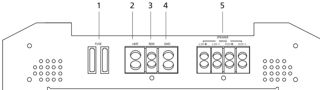
1. **ATC Fuse** - (2) 30-amp ATC fuses protect the amplifier against internal electrical damage and is meant to protect the amplifier only. All other power connections should be fused at the source.
