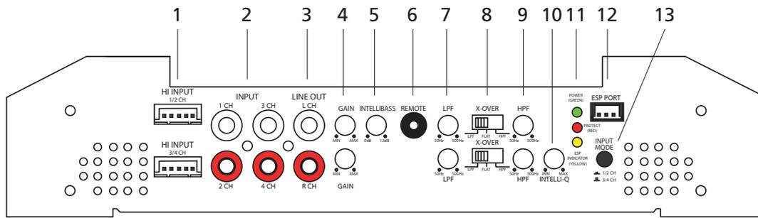
1. **Hi Input** (high level input Ch 1/2 and Ch 3/4) - Accepts 1v to 10v input from the head unit's speaker output. The amplifier will automatically wake-up when the input is greater than 1V (on channel 1/2 high level input only).
