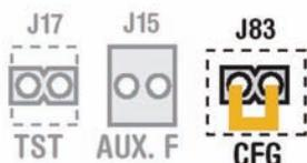
When the logic jumper is installed on J83 (CFG), configuration settings are enabled. DIP switches will then operate as shown below.
