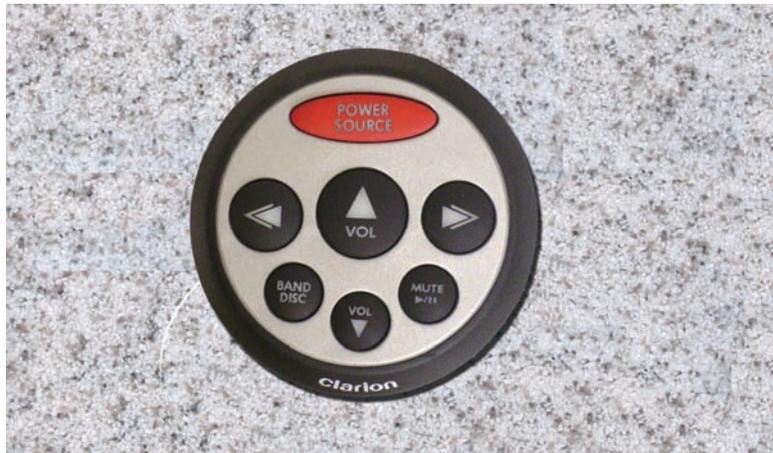
**Figure 29. Clarion topside mounted remote control**
