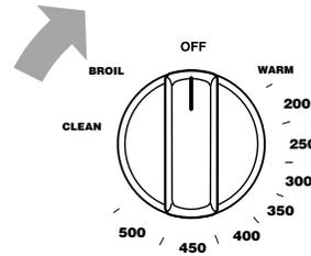
**YOU SEE DOOR LOCKED/ CLEANING light stays on. COOL appears in display until oven goes below locking temperature.**
