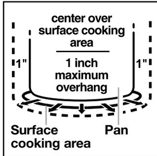
cooking area. Large diameter canners/pans, if not centered correctly, trap heat and can cause damage to the cooktop.
