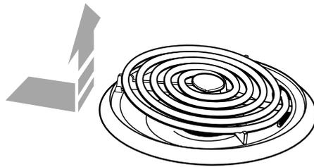
3. Pull the coil element straight away from the receptacle.
