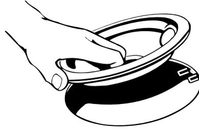
3. Hold the coil element as level as possible with the terminal just started into the receptacle. Push the coil element terminal into the receptacle.
