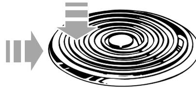
**NOTE:** Reflector bowls reflect heat back to the cookware on the coil elements. They also help catch spills. When they are kept clean, they reflect heat better and look new longer.
