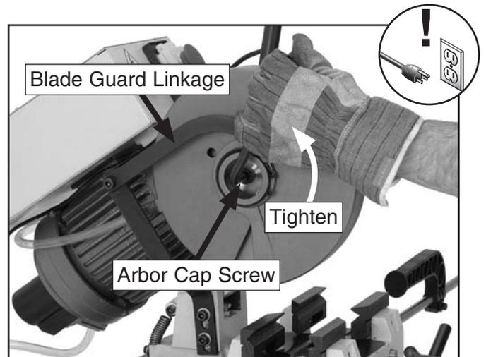
**Figure 26.** Tightening blade.
