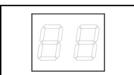
**Digital Load Meter (Ammeter):** The total electrical current used by the PDU is displayed on the digital meter in amperes.
