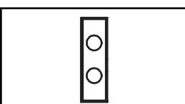
**Input Source Indicator:** When the PDU is connected to a live AC power source, the Primary or Secondary input LED illuminates to indicate which source is supplying power to the PDU outlets.
