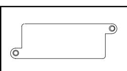
**Accessory Slot:** An optional SNMP card may be installed in the slot, allowing the PDU to be configured, controlled and monitored remotely. Contact Tripp Lite Customer Support at (773) 869-1234 for more information.
