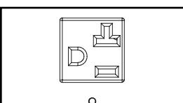
**NEMA 5-15/20R Outlets (Model PDUMH20AT):** During normal operation, the outlets distribute AC power to connected equipment. When an outlet is live, the associated LED illuminates.
