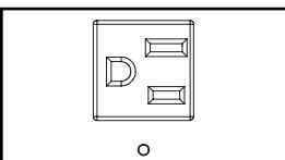
**NEMA 5-15R Outlets (Model PDUMH15AT):** During normal operation, the outlets distribute AC power to connected equipment. When an outlet is live, the associated LED illuminates.
