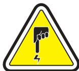
DO NOT TOUCH the print head or the electronic components on the print head carriage. Discharges of electrostatic energy that accumulates on the surface of the human body or other surfaces can damage the print head and other electronic components used in the device.
