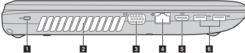
**1 Kensington slot** Attach a security lock (not supplied) here.
