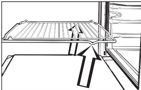
The racks have non-tip safety notches which prevent them from being pulled out completely while the oven is in use.
