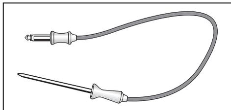
The roast probe reliably monitors the core temperature of meat and poultry during a roasting function.
