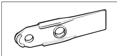
Use the slide opener to remove the light cover.
