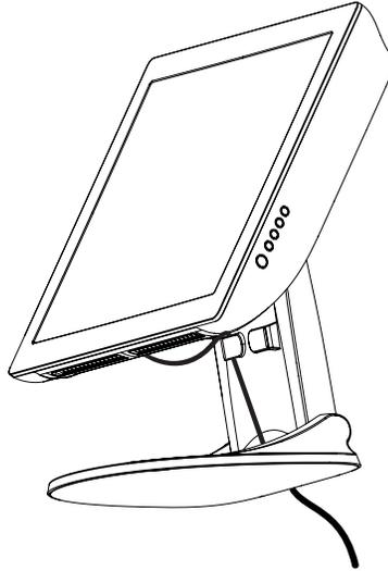
**NOTE** Before connecting the cables to the touchmonitor, route all the cables through the hole in the second as shown in the picture above.
