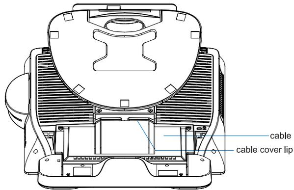
Then you have attached all the cables to the monitor, gently bring all the cables toward the standard so they fit under the cover lip.
