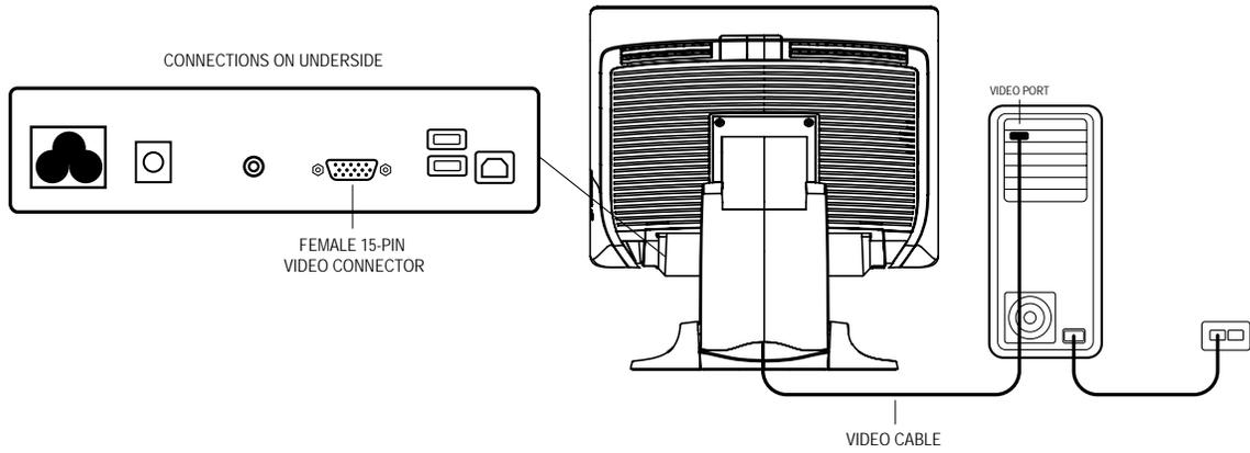
Connect one end of the **video cable** to the rear side of computer and the other to the LCD. Tighten by turning the two thumb screws clockwise to ensure proper grounding.
