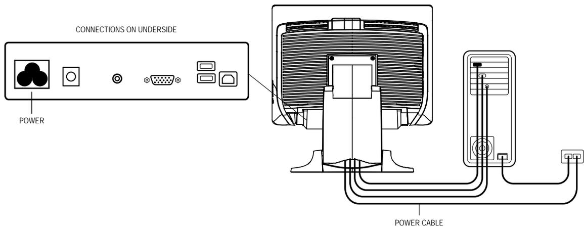
Connect one end of the **power cord** to the monitor and the other end to wall.
