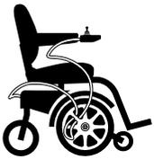
Use correct tie-down points for controller harness to prevent the harness from getting caught in the drive tires or pinched in the seat frame.
