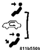
Select the recirculation modes when the outside air contains dust, odors, high humidity, or if rapid cooling is desired. This feature allows for recirculation of interior air only. Air flows through either the panel outlets or both the panel and floor outlets, together, depending which recirculation mode is selected.
