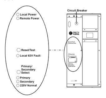
**Circuit Breaker:** The circuit breaker protects the 220 V input from overload conditions.
