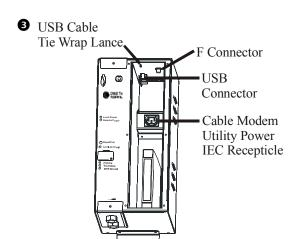
Connect the appropriate cables to the cable modem IEC receptacle, the USB port, and the F-connector located on inside the enclosure.
