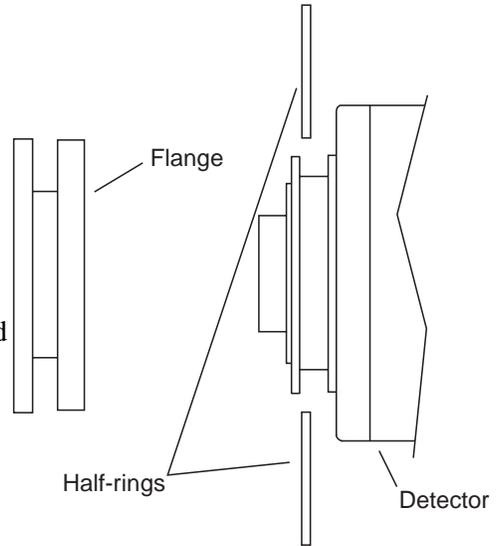
Figure 5. Shallow Focal Plane Spectrograph Mounting Hardware
