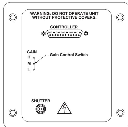
Figure 2. NTE Detector Rear Panel
