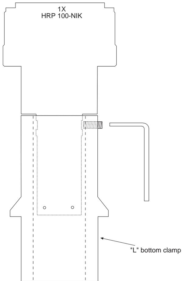
Figure 12. Bottom Clamp Secured to Relay Lens
