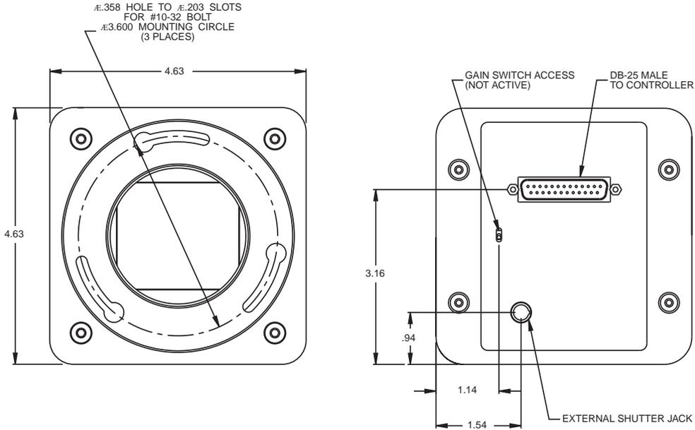
Figure 16. Spectrometer Mount: Front and Back View
