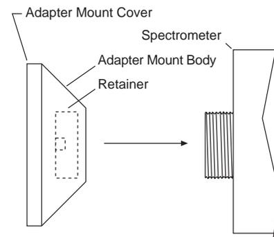
Figure 6. One Type of Entrance Slit Shutter Mount
