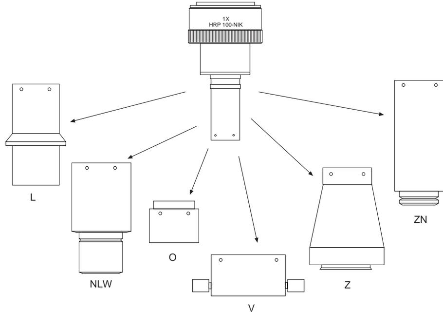
Figure 11. Diagnostic Instruments Bottom Clamps for Different Microscopes
