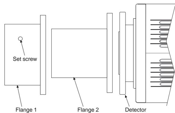
Figure 4. Adapter for a Deep Focal Plane Spectrograph
