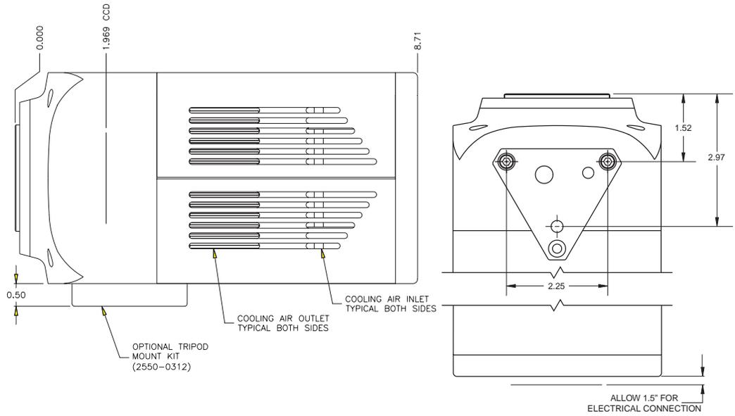
Figure 21. Fiber Optic Coupled: Side and Bottom Views
