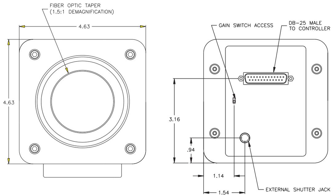
Figure 22. Fiber-Optic Coupled: Front and Back View
