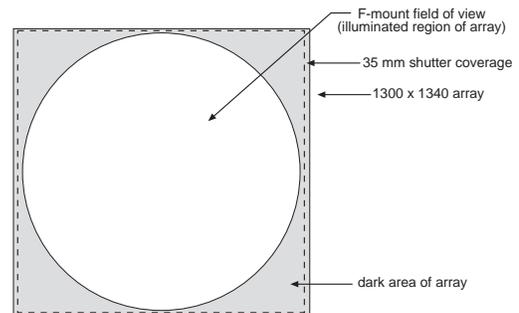
Figure 13. Coverage on 1300×1340 Array for F-mount Design
