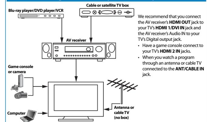
We recommend that you connect the AV receiver's **HDMI OUT** jack to your TV's **HDMI 1/DVI IN** jack and the AV receiver's Audio IN to your TV's Digital output jack.
