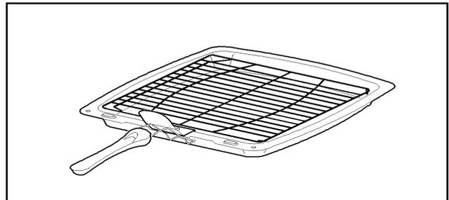
To remove the handle, slide the handle to the right and lift the handle away from the cut out on the grill pan.
