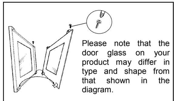
3. Hold the door glass securely in place with one hand before removing the screws completely with the other hand.
