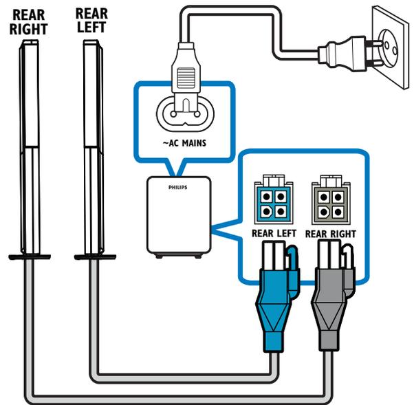
Connect the rear left and rear right speakers to the matching connectors at the back of the wireless receiver.
