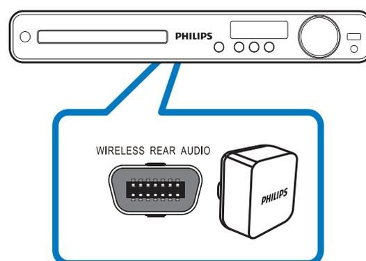
Connect the wireless transmitter to the **WIRELESS REAR AUDIO** connector on the back of the home theater.
