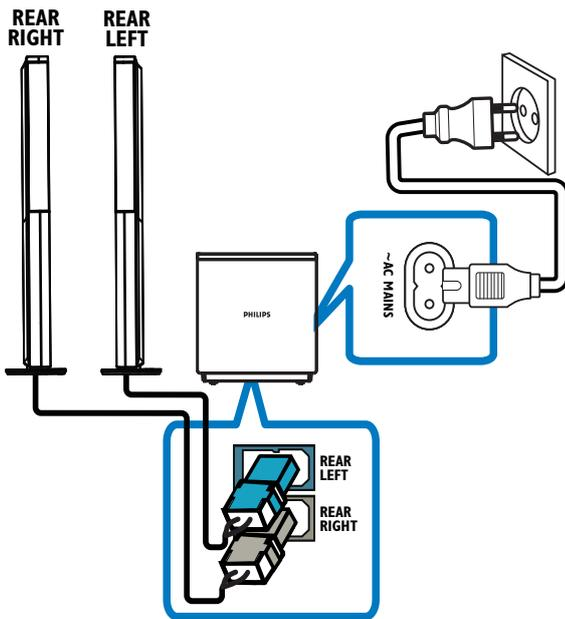
Connect the rear left and rear right speakers to the matching connectors at the bottom of the wireless receiver.
