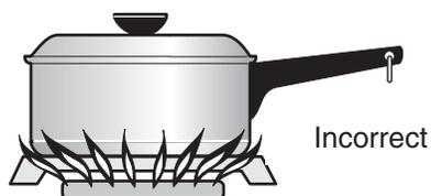
Never extend the flame beyond the outer edge of the utensil. A higher flame simply wastes heat and energy, and increases the risk of being burned by the gas flame.
