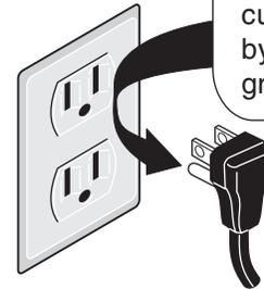
Do not, under any circumstances, cut, remove, or bypass the grounding prong.
