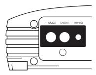
The e2150's "+12VDC" and "Ground" connections are designed to accept 8 AWG - 4 AWG power wire. 8 AWG is a minimum power wire size for this amplifier.
