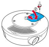
Align the lamp cover, and press it in, then tighten the screws loosened in Step 4 until the lamp cover is no longer loose.
