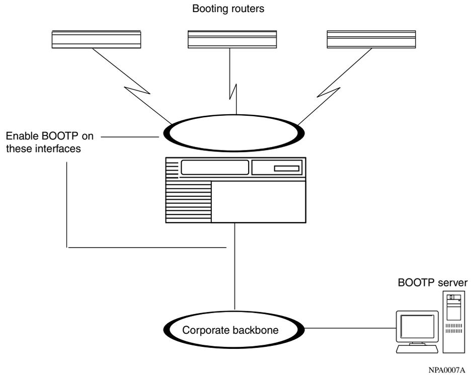
**Figure 3-1. Enabling BootP Relay in a Sample Network**
