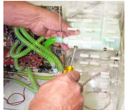
Figure 6: Once full, secure the reservoir to the drive-bay with the provided screws. Installation is complete!
