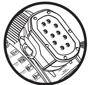
**Note:** The 9.6 Volt, 12 Volt, and 14.4 volt battery packs will not slide all the way down onto the charger port. Insert 9.6 Volt, 12 Volt, and 14.4 Volt battery packs until they click into place and are aligned with the line on the charger, shown at left.
