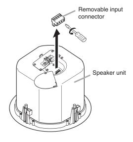
**Step 3.** Insert the stripped cable end into the terminal and tighten the terminal screw with a screwdriver.
