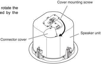
**Step 2.** Detach the removable input connector from the speaker's socket, and loosen the screw of the terminal to be used.
