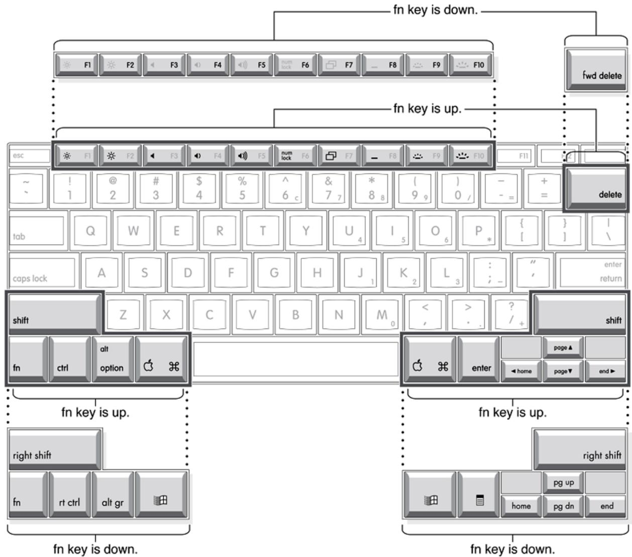
Figure 3-8 Embedded numeric keypad operation
