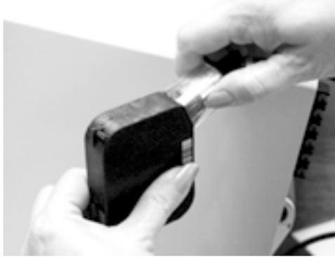
5. Channel hose attached to bulk ink cartridge to clips on printer as shown.
