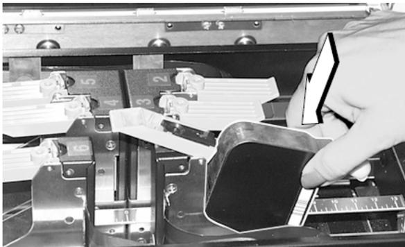
5. With the gold printhead contacts pointing toward the printhead holder pins, fully insert the cartridge into the holder. **DO NOT** contact or bend the printhead holder pins.
