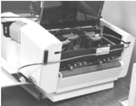
6. Insert printhead cartridge into holder.
