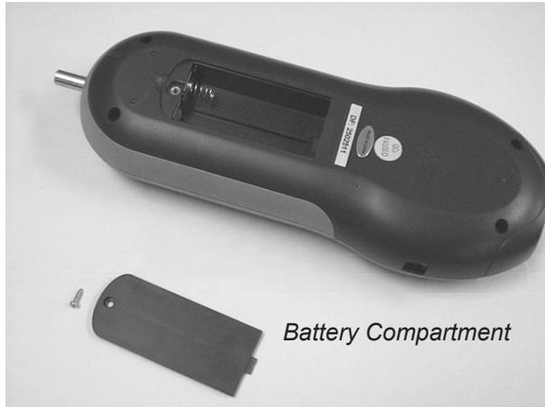
1. Before use, install (4) 1.5 VDC "AA" batteries (not supplied).
