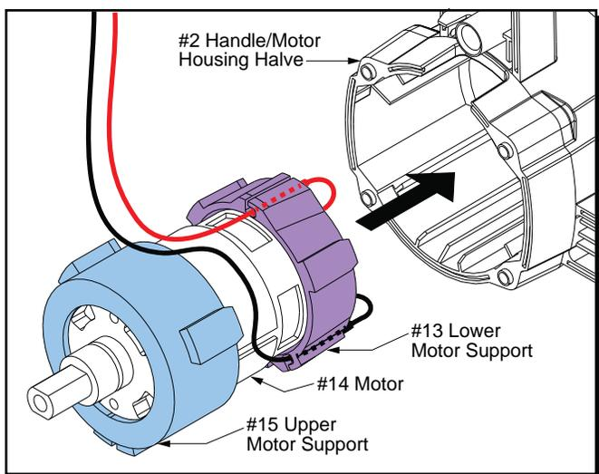
When reinstalling a new Motor Assembly, be sure that the red and black motor leads are fed through the large opening in the back of the Lower Motor Support before soldering wires to the On-Off Switch.
