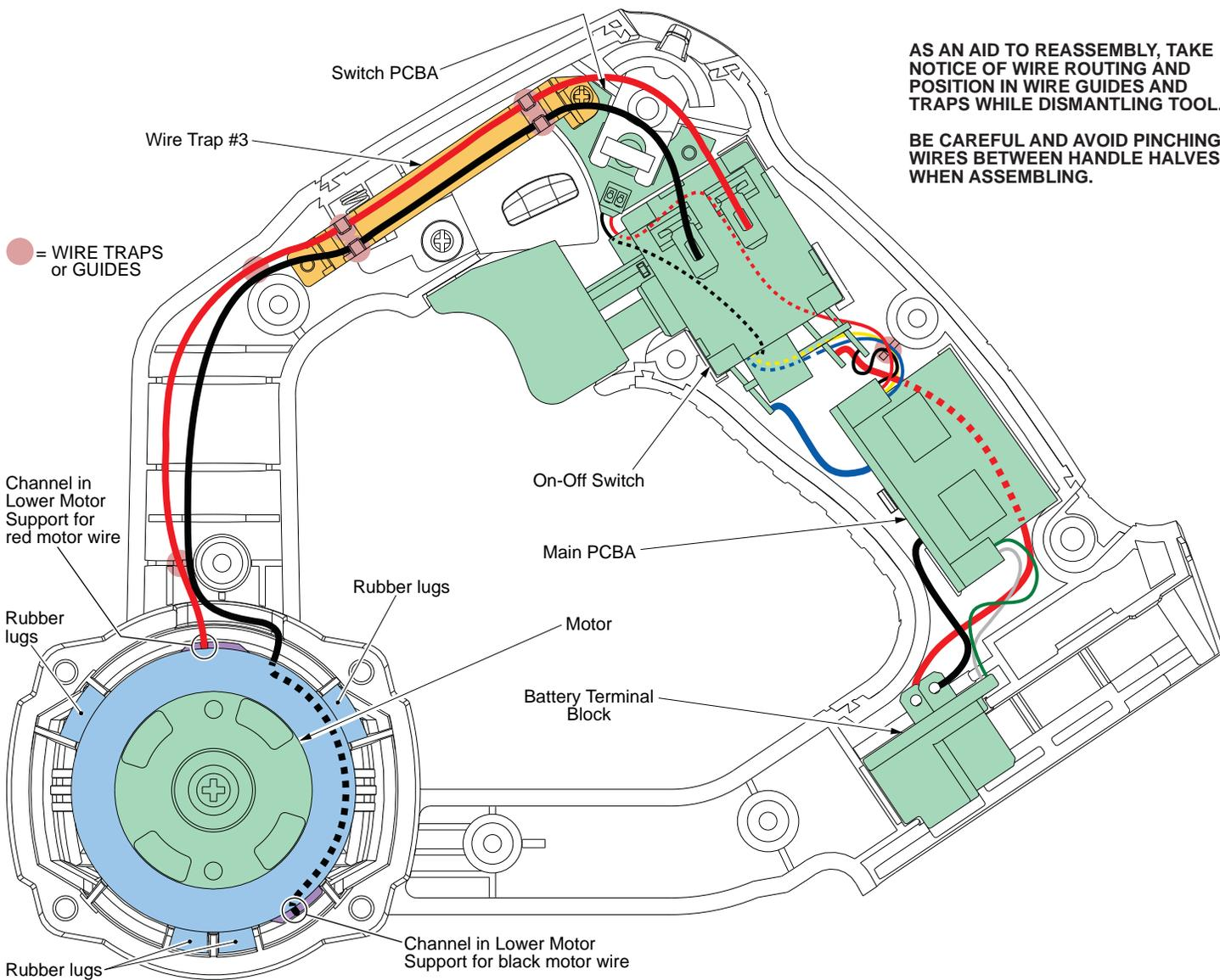
AS AN AID TO REASSEMBLY, TAKE NOTICE OF WIRE ROUTING AND POSITION IN WIRE GUIDES AND TRAPS WHILE DISMANTLING TOOL.
