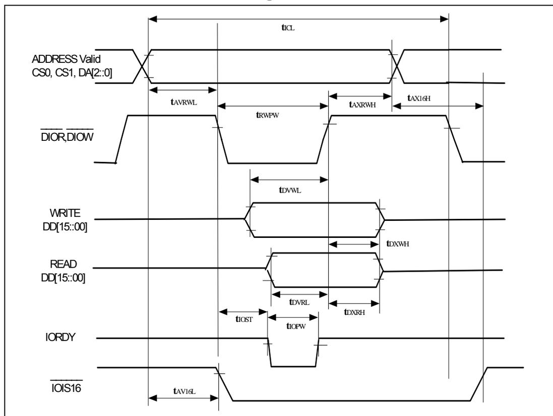
Figure 6: True IDE Read/Write Access Timing Diagram
