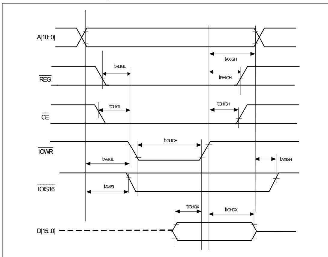
Figure 5: I/O Access Write Timing Diagram
