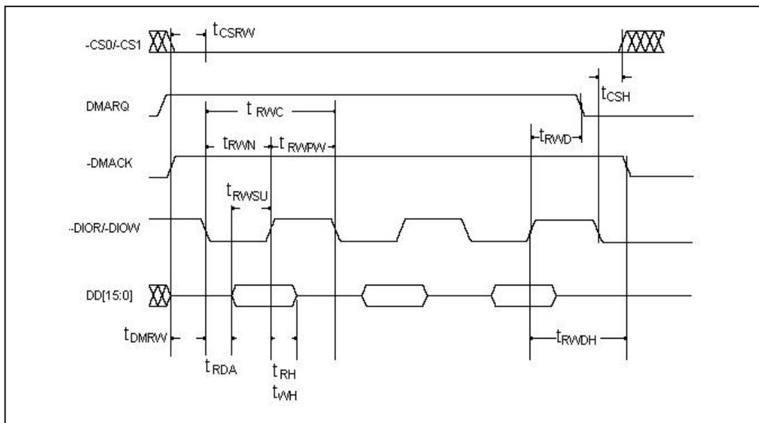
**Figure 7: True IDE Multiword DMA Read/Write Access Timing**
