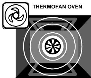
**4** The rear bake element is used in conjunction with the fan.
