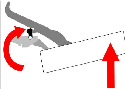
Flip the retainer clasps up and over the hook on the upper hinge arm .
