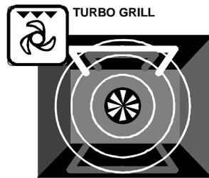
**5** The top grill element is used in conjunction with the fan.
