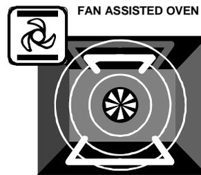
**3** Top heat and bottom bake elements are used in conjunction with the fan.
