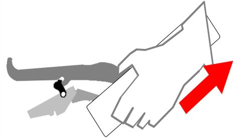
Lift the door upwards and outwards until it is free of the hinge housing
