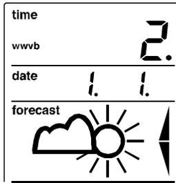
5. Press and release the *IN* button to select the forecast sensitivity
