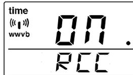
5. Press and release the *IN* button to select radio-controlled time on or off.
