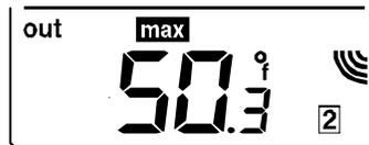
3. While “MAX” is still displayed press the *OUT* button again to return to the current data display. Or you can wait 30 seconds, during either the minimum or the maximum readings, and the unit will automatically return to current data readings.
