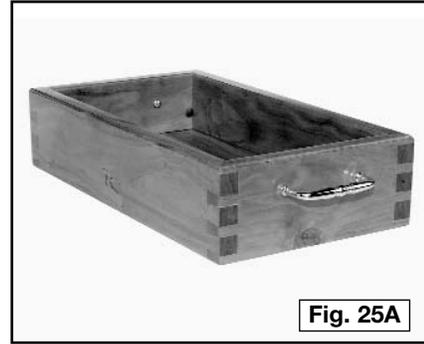
**NOTE:** Depending on the depth of the molded edge, you may want to make the boards slightly wider to account for the molded depth. If so, mount the tail board so that the mitered edge will end with the thicker half-pin. With the offset guide set against the tail board, the pin board will automatically be cut correctly.
