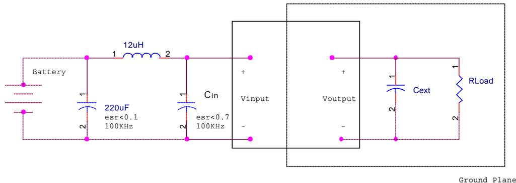
The input reflected ripple is measured with a current probe and oscilloscope. The ripple current is the current through the 12uH inductor. The capacitor Cin shall be at least 100uF/100V. One 470uF or two 220uF/100V capacitors in parallel are recommended.
