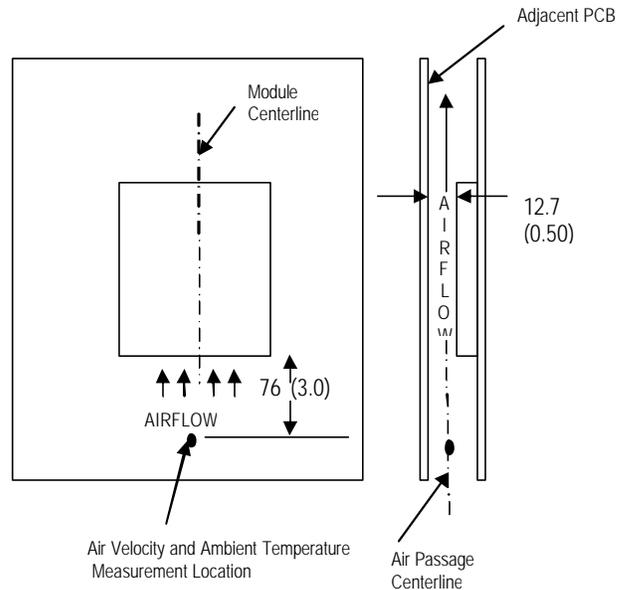
**Wind Tunnel Test Setup Figure**
