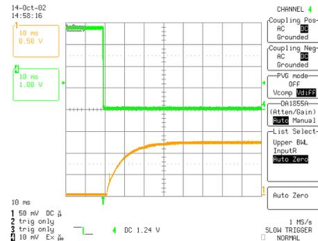
iHA48060A012V-001 Typical startup characteristic from on/off at full load. Upper trace - on/off signal, lower trace – output voltage
