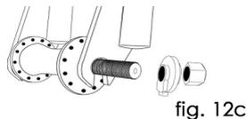
adjustable wrench, loosen the two axle nuts.
