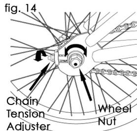
d. Push the wheel forward to slacken the chain, and remove the chain from the chainring and wheel sprocket.
