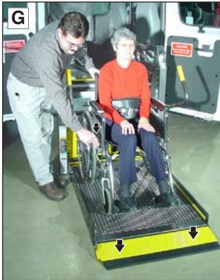
◀ **Note:** Passenger **must** be positioned **fully inside yellow boundaries**. ▶
