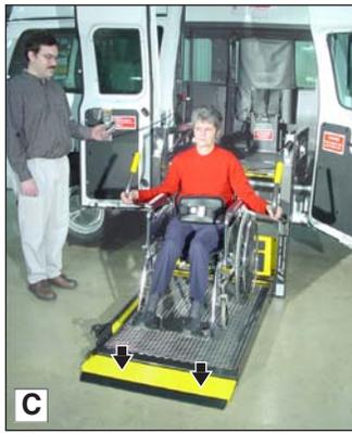
3. Unlock wheelchair brakes and unload passenger from platform. ▶
