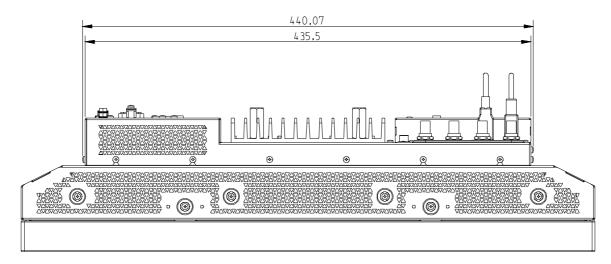
Figure 63: RHDM-2301 Top view (metric units (mm))
