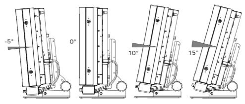
Figure 72: Variation of angles that can be reached with the tiltable stand
