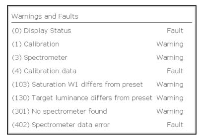
This menu lists all faults and warnings which have occurred. When a fault occurs, the "FAULT" LED on the control panel and the "Cal/Err" LED on the bezel will light up red.
