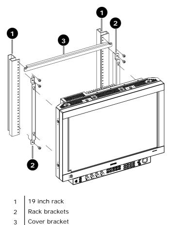
Figure 76: Rack mounting of the display unit
