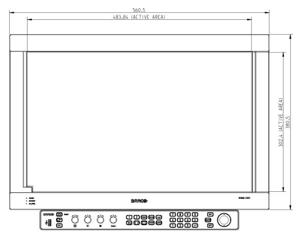
Figure 62: RHDM-2301 Front view (metric units (mm))
