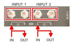
Figure 10: Input connectors SDI input board
