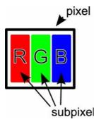
Figure 60: Pixel and subpixel definition
