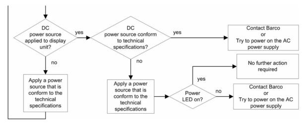
Figure 81: "No power" fault finding tree
