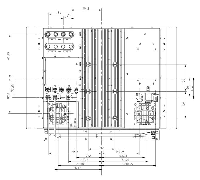
Figure 64: RHDM-2301 Rear view (metric units (mm))
