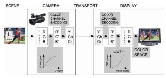
Figure 52: From captured light on the scene to the image on the screen
