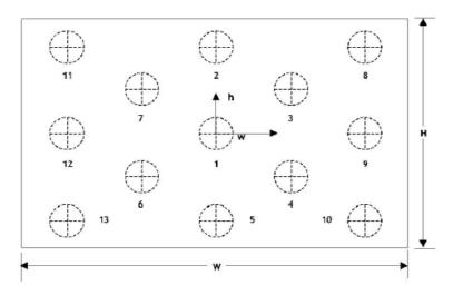
The area of measurement is not greater than a circle of diameter 0.1H.
