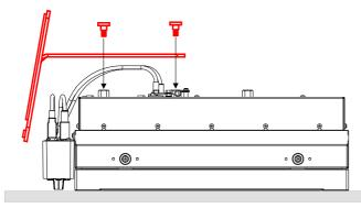
Figure 70: Mounting of Barco stand – screw location
