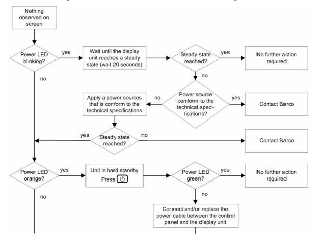
7.10.4 "Nothing observed on the screen" fault finding tree
