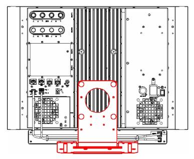
Figure 71: Mounting of the Barco stand - rear view
