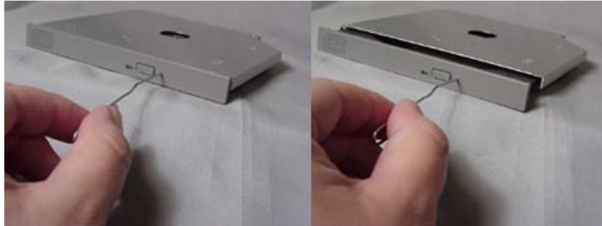
**Figure 2.Using Emergency Eject**
