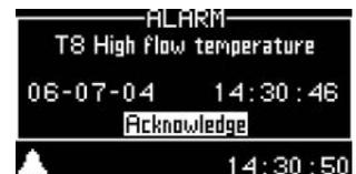
**Possible cause 2:** Particle filter is clogged.
