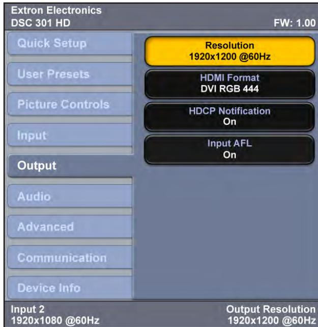
**Figure 8. OSD Menu – Output Submenu**
