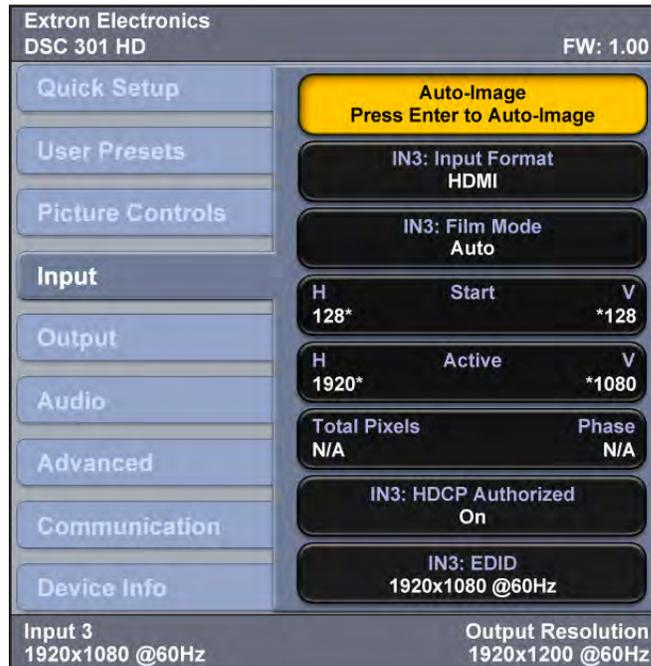
**Figure 7. OSD Menu – Input Submenu**
